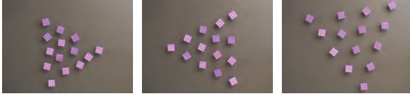
Fig. 18. Dynamic image display, with 14 e-puck robots show a continuously rotating and enlarging triangle. The full video is available as Extension 1.
