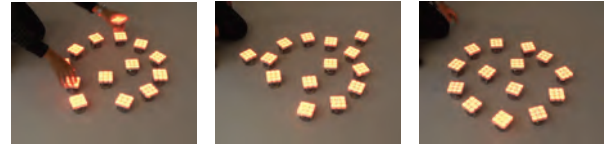
Fig. 20. Perturbation recovery, with 14 e-puck robots form a rotating disk pattern. Two of the robots are picked up and placed outside the disk. The formation recovers and the two robots are incorporated smoothly back into the disk. The full video is available as Extension 1.
