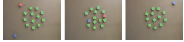
Fig. 19. Dynamic obstacles. The green robot pixels are part of the normal display and are showing a static disk pattern. The red and blue robots are uncontrolled objects moving through the workspace. The green pixels respond in order to avoid collision with the dynamic obstacles. The full video is available as Extension 1.
