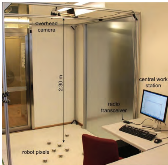
Fig. 10. The system consists of a group of differentially driven robot pixels, an overhead camera, and a standard PC with radio module.
