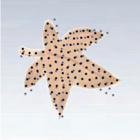
Fig. 9. Goal positions (black circles) for 100 robots representing the leaf of the animation of Section 7. The initial samples (blue stars) were obtained from the previous keyframe, using an estimate of the translation and rotation of the global shape.
