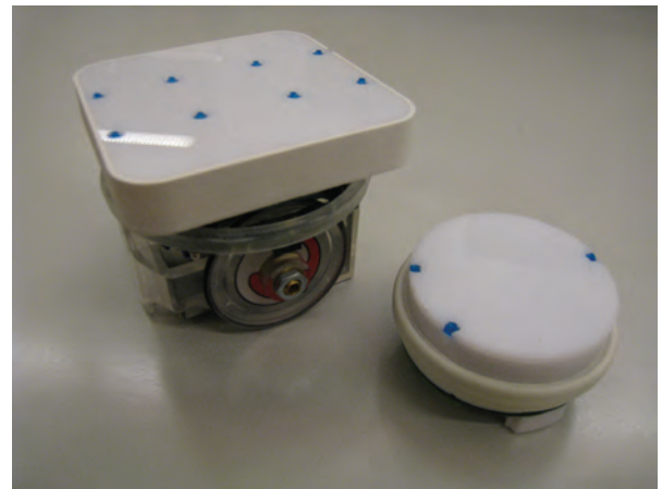
Fig. 11. Robot pixels. At left, the modified e-puck robot with a 3 \times 3 RGB LED array. At right, the Elisa robot with a single RGB LED (see Section 7.5.1). The blue spots are infrared LEDs.
