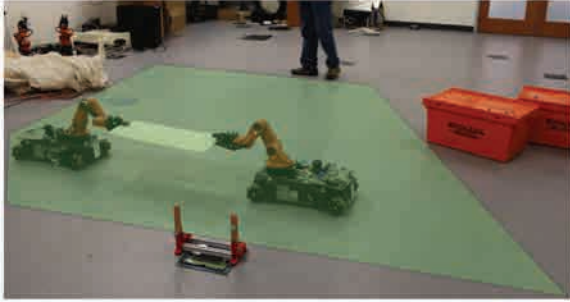
Fig. 1. Two mobile manipulators collaboratively carry a rigid object. A projection of the obstacle-free convex region is superimposed in green.
