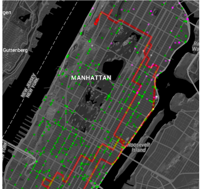
Fig. 1: A snapshot of the simulator. Green dots represent vehicles that either have passengers on board or are on their way to pick up passengers. Pink dots represent vehicles that are rebalancing. Grey dots represent vehicles that are idle. The snapshot furthermore shows the location and history of one of the vehicles in the fleet (represented by the red car).
