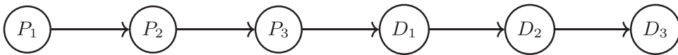
Figure 1. An illustrative itinerary of a vehicle serving a shared ride for three passengers, that are first picked up at their origins and then dropped off at their destinations.
