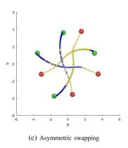
Fig. 2: Simulation results for each scenario using our communication policy. Solid lines represent the trajectories executed by the drone-swarm. Yellow represents the positions where the drones communicate their trajectory plans. Blue depicts the positions where the drones do not communicate. Green and Red represent the initial and goal position of each drone, respectively. Increasing opacity represent the episode progression.
