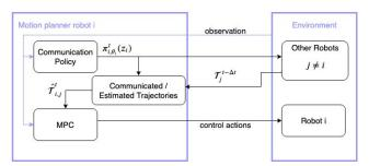
Fig. 1: Schema of the proposed method for efficient communication.  $\pi_i^t(z_i)$  is the communication policy dependent on the observation  $z_i$ .  $\mathcal{T}_j^{t-\Delta t}$  is the trajectory plan of robot j at the previous time step. And  $\hat{\mathcal{T}}_{i,j}^t$  are the combination of obtained and estimated trajectories of the other robots.
