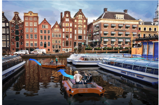
Fig. 1: A visualization of two Roboats navigating Amsterdam’s canals. The blue arrows represent their planned motion. ©MIT/AMS Institute.
