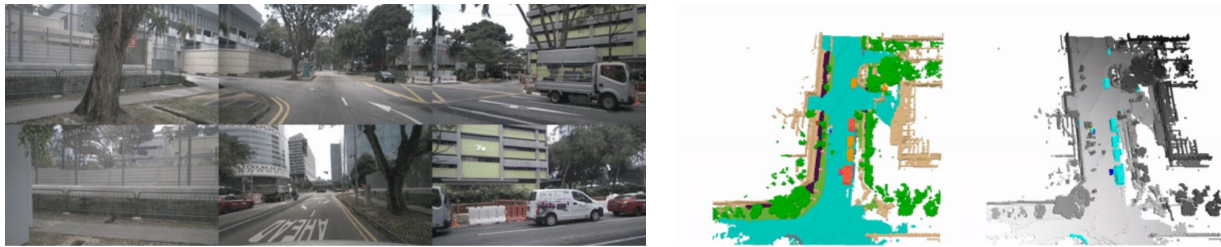
Fig.1. Occupancy Prediction in Autonomous Driving [1]. The left side shows the images captured by the cameras around the vehicle. The right side shows the predicted occupancy map with different colors suggesting different semantic labels.
