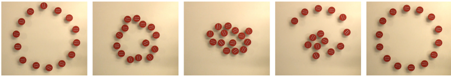
Fig. 5 Experiment 2 with fourteen e-puck robots. The sequence shows collision-free transition of the e-pucks through the circle center to the antipodal position on the circle's boundary.
