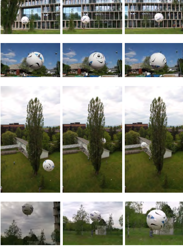
Fig. 10. Qualitative results obtained for outdoor deployment. (a) Translation at 20km/h. (b) Rotation at 0.5 rev/s. (c) Circumnavigating a tree. (d) Safe and easily-deflected contact with a human.
