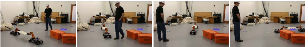
Figure 12. Four consecutive snapshots of an avoidance maneuver where two mobile manipulators collaboratively carry a rigid object and navigate it to the goal while adjusting their formation to avoid collisions with the orange boxes and the human. Robots and human are tracked by overhead cameras. This maneuver is performed in 1 minute.
