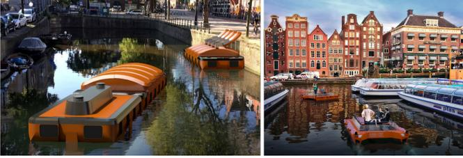
Fig. 1. Roboat: Robotic boats designed to serve as a platform for trash removal and as a new means of transportation in Amsterdam canal.
