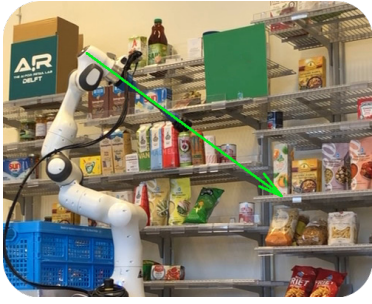
Fig. 9: Illustration of the orientation constraints for trajectory generation for look-for-product.
