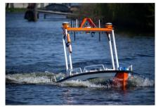
Autonomously sailing on open waters is a challenging task, especially in adverse weather. The motion planner guiding the vessel has to be robust to disturbances, e.g. wind and currents, which are inherently stochastic.
