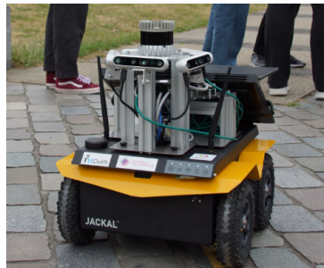
Fig. 1 Jakal Mobile Robot with RGB-D Cameras and Lidar
