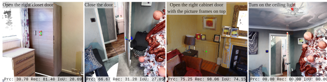
Fig. 2. Qualitative examples of T-FunS3D. We visualize point clouds around the functional components: red points indicate predictions, blue points denote ground truth, and green points represent overlaps.
