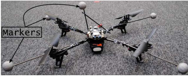
Figure 6: The quadrotor used in the tests with a focus on the VICON passive markers used to track it through the VICON system.
