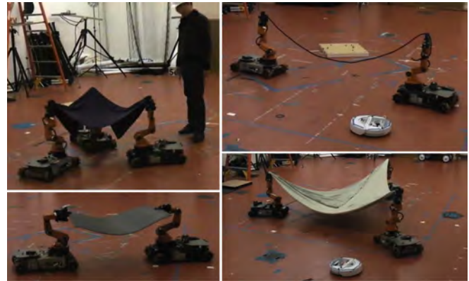
Fig. 7. Collaborative manipulation of deformable objects. Mobile manipulators carry the object while avoiding static and dynamic obstacles.
